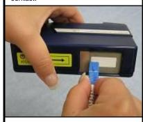
**Step 3:**Release the lever to close shutter
